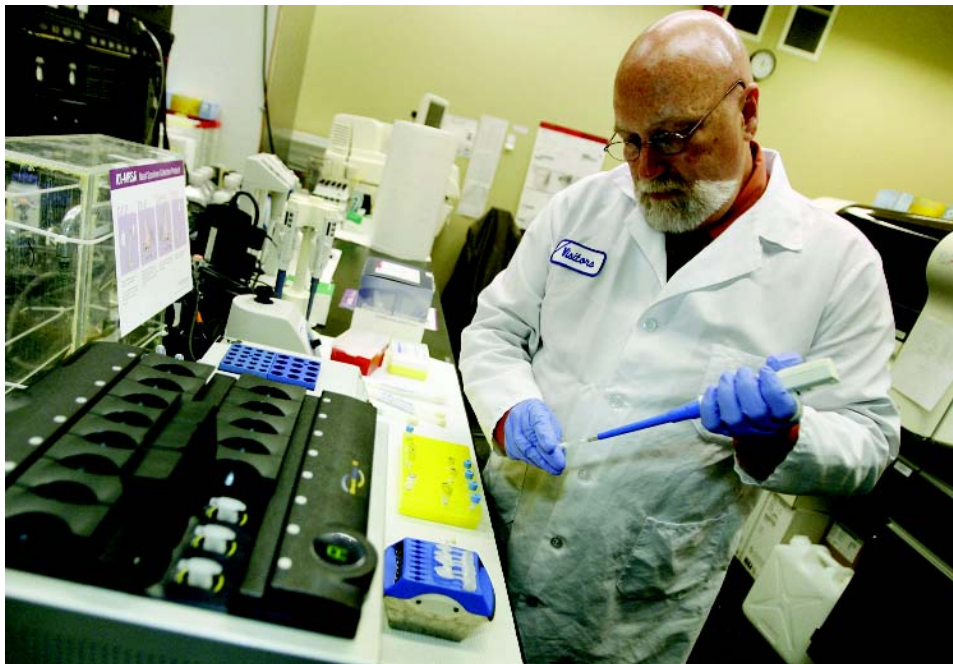
A technician loads patient samples with PCR reagents into a thermocycler, which heats and cools the samples and amplifies the DNA. Using fluorescence, the instrument then detects the resistant organism in the sample. The results are sent to a computer. © Jerry McCrear/Star Ledger/Corbis.
